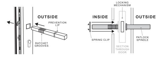
Hold the Patlock spindle firmly from the outside and push the spring clip onto the Patlock spindle from the inside of the door ensuring that the clip engages with the grooved section to secure in position. Increase the hole in the door casing if required to ensure the spring clip fits against the locking mechanism.
